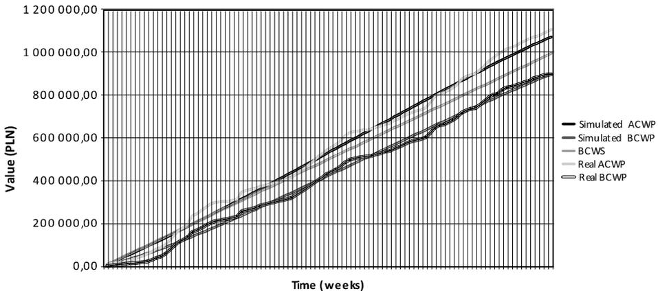
**Figure 2.** Comparison of the results generated by the simulation to the real project data
